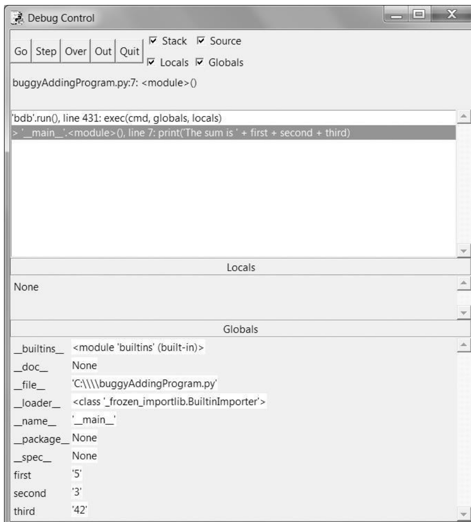
Figure The Debug Control window on the last line. The variables are set to strings, causing the bug.
