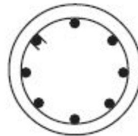
Fig. 5.3 : RCC square and circular columns with steel reinforcements
